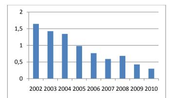
Figure 1: The annual number of ships on collision course, divided with the number of platforms surveyed. All the data are observed from Sandsli Maritime Control Centre. The figure is made from data collected by Jan Erik Vinnem (PSA, 2011).
