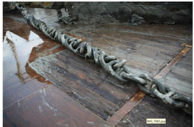
Figure 9: Twisted chain on the deck of an anchor handler vessel (Norland et al, 2012).
