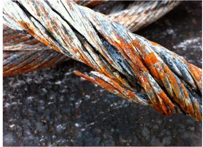
Figure 6: Representative picture of failed single wires, and on corrosion on a strand after two years in use (DNV, 11.3.2012).
